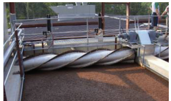
DAFF with hydraulic sludge decanting
